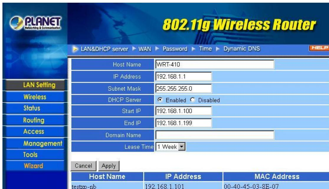
This page enables you to set LAN and DHCP properties, such as the host name, IP address, subnet mask, and domain name. LAN and DHCP profiles are listed in the DHCP table at the bottom of the screen.
